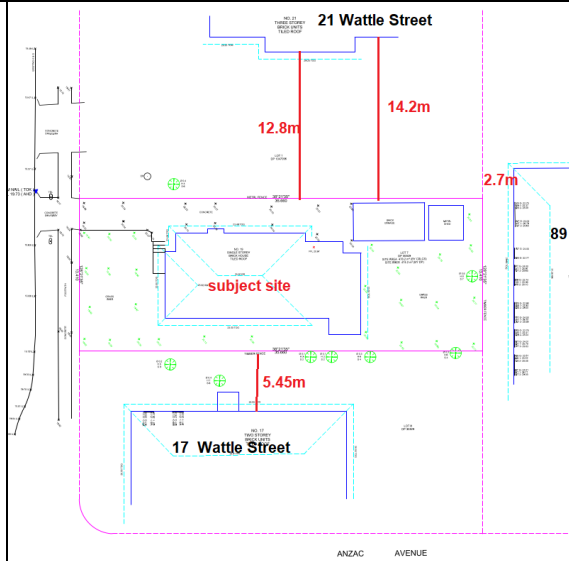
Figure 15: Site plan of site illustrating the setbacks/location of adjoining buildings.
