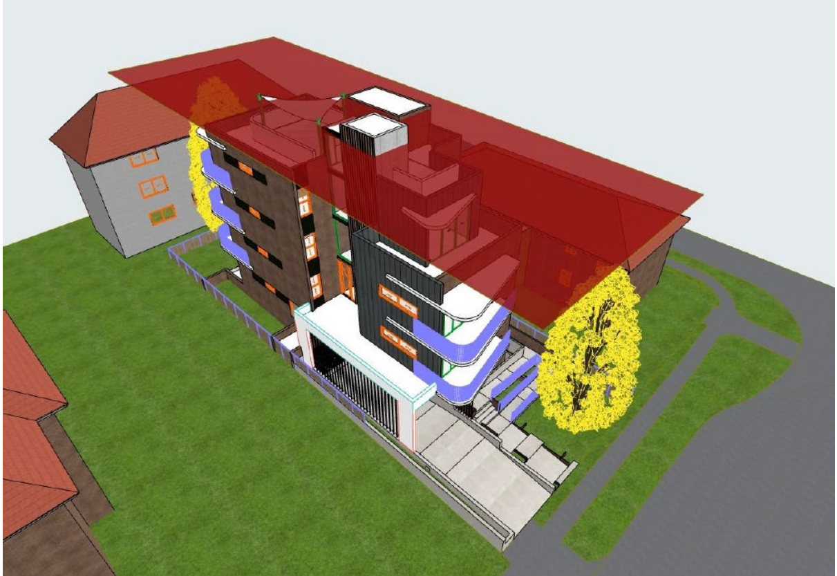
Figure 17: Height plane showing the extent of non compliance to the lift well and also for small section of the fire stairs, corner tips of the shade cloth, relative to the height limit.
