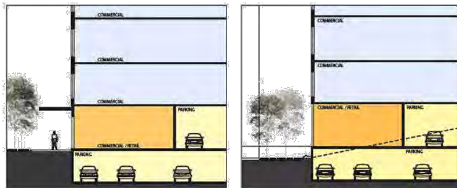
Figure 8.6.3 Along Active Frontages, basement parking must be located fully below footpath level. However to accommodate topography, basement levels may protrude by a maximum of 1.2 m beyond ground level. Along street frontages, above ground parking must be laminated with another use.
