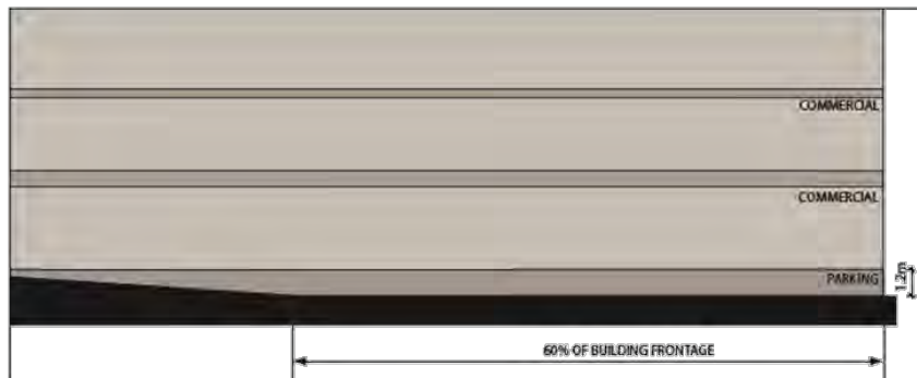
Figure 8.6.2 Along public streets, basement parking must protrude no more than 1.2 m above ground for no more than 60% of the building frontage.
