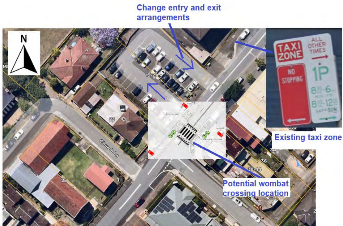
Figure 1 – Aerial view showing potential wombat crossing location and existing taxi zone
