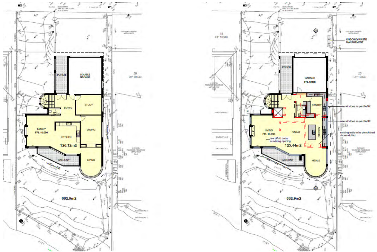
Figure 9: Proposed ground floor plan with existing plan on the left and proposed on the right.
