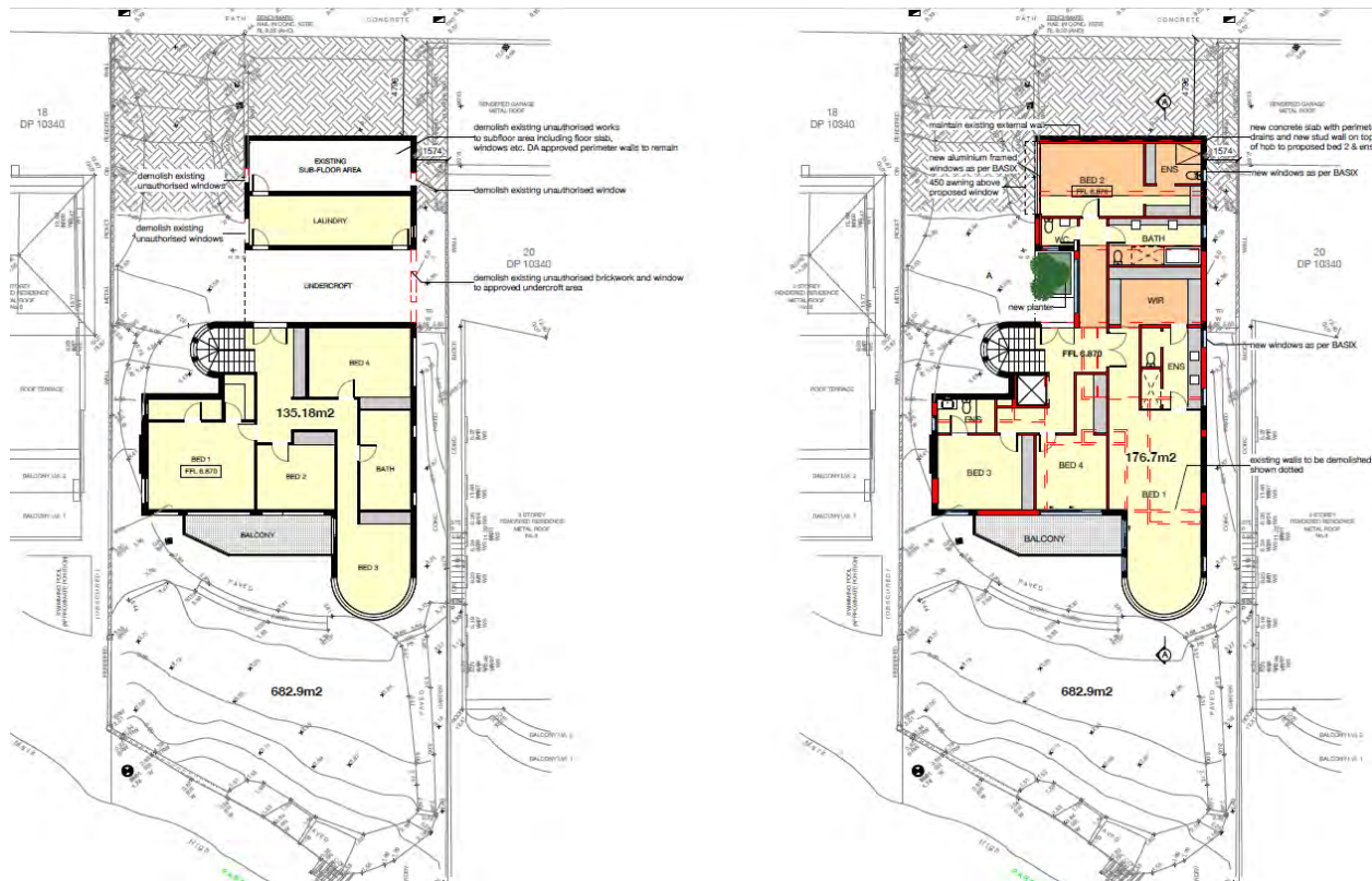
Figure 8: Lower ground floor plans with existing floor plan on left and proposed on right.
