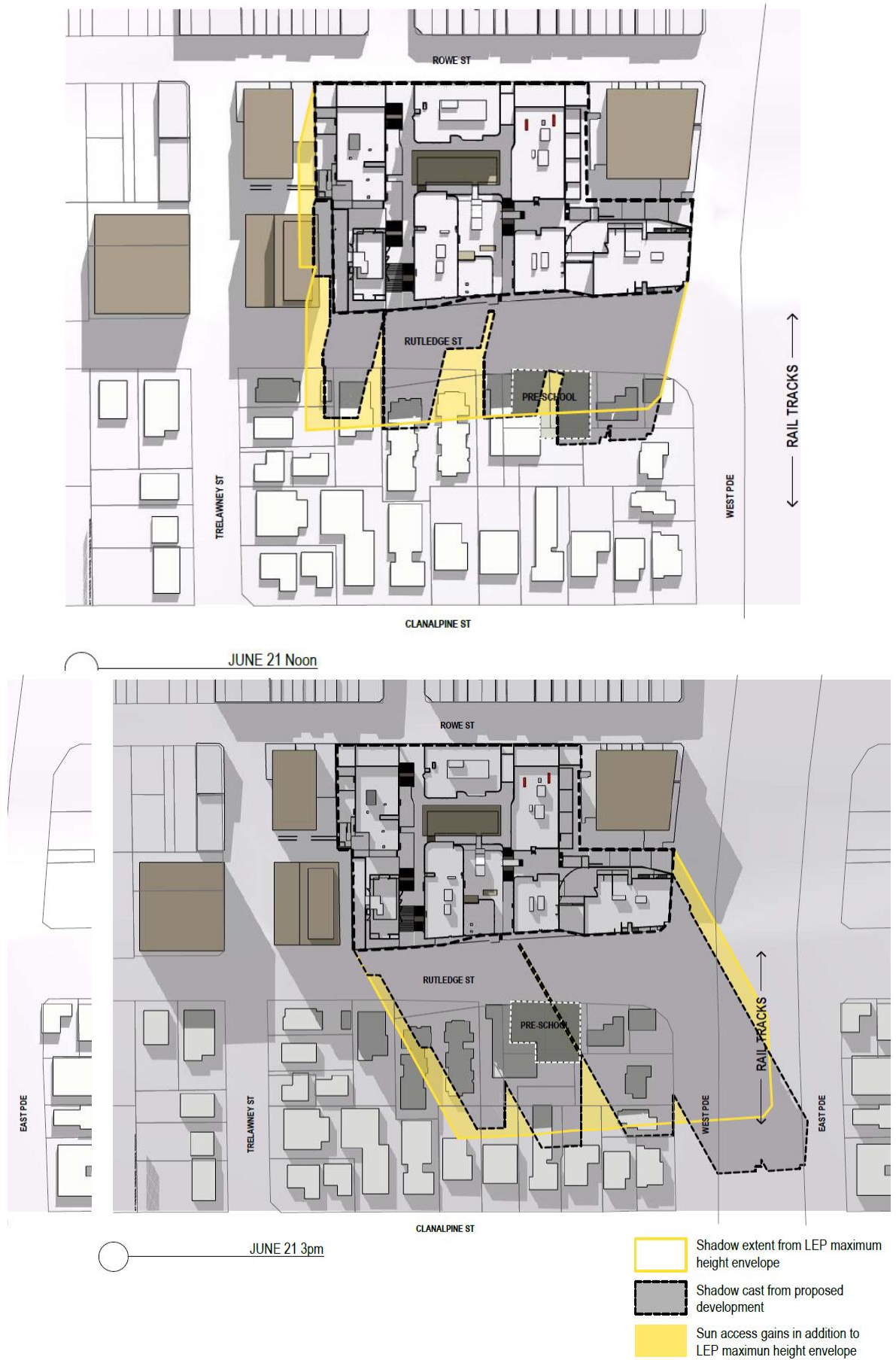
Figure 27: Shadow diagrams showing shadow extent, LEP maximum and solar gains through alternate design
